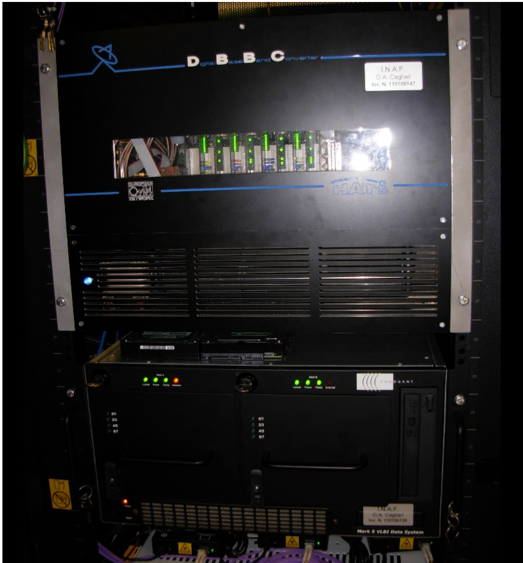
Figure 6: DBBC & Mark5C at the Sardinia Radio Telescope apparatus box
