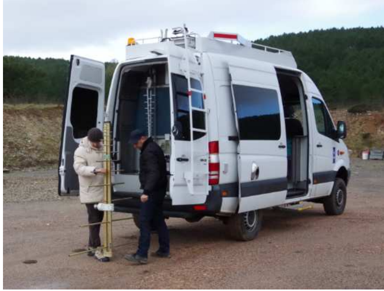
Figure 1: The Log periodic LPA 360-6 antenna is prepared to be mounted at the mobile laboratory.
