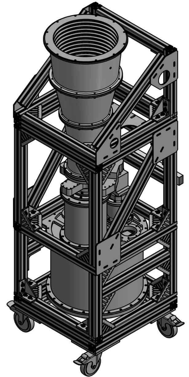
⊕ It is required to make at least 4 calibrated holes suitable to accommodate the Retroreflector supports for the LaserTracker 0.5 ", these holes must have known coordinates.
