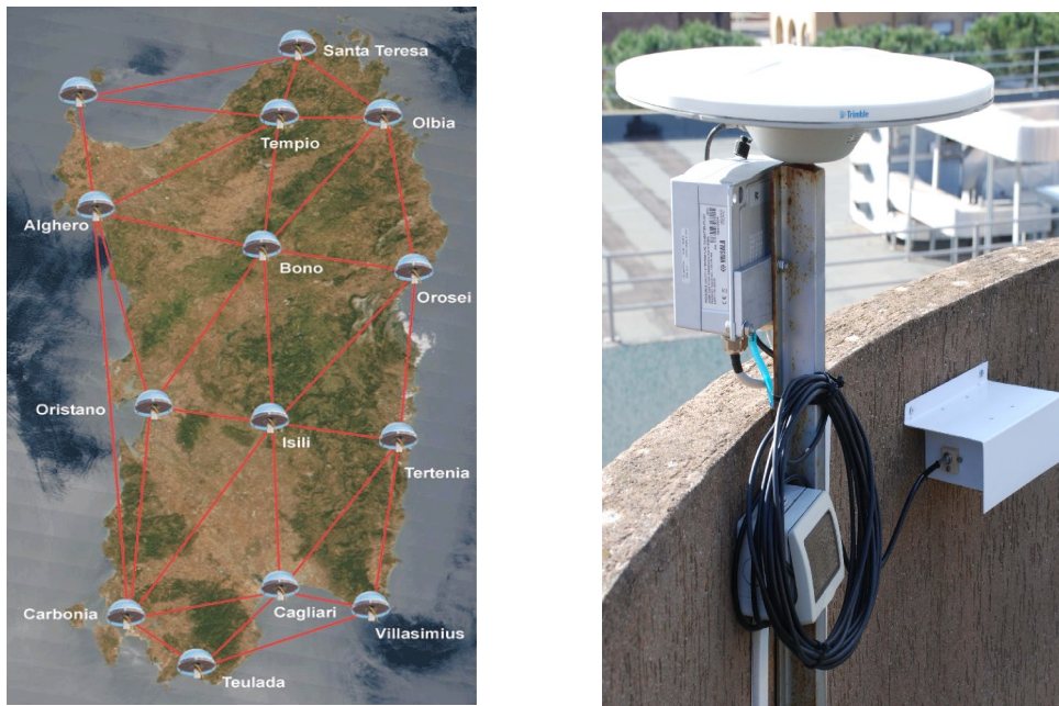
Figure 1: (left) The SARNET network stations located in various cities of Sardinia (ITALY). (right) A trimble geodetic GPS receiver placed in one of the locations on the map next to a Vaisala meteorological surface station.
